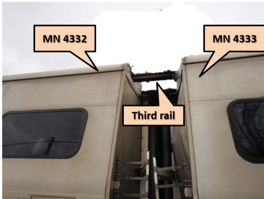
Figure 17. Third rail between railcars Metro-North 4332 and 4333.
