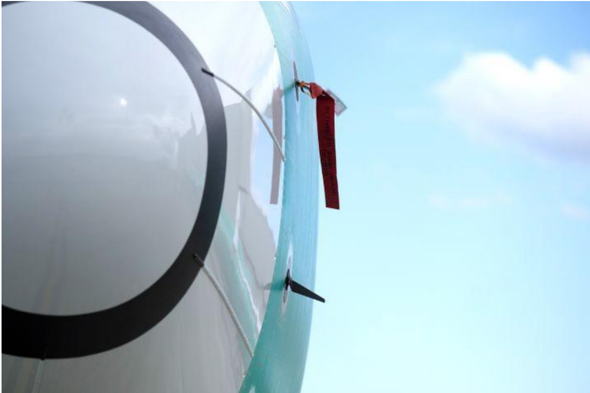
One of two sensors that measures the angle of attack is pictured at bottom on a Boeing 737 MAX 8 airplane outside the company's factory: Boeing appears to have ignored the vital rule of redundancy. Stephen Brashear / Getty Images / AFP
