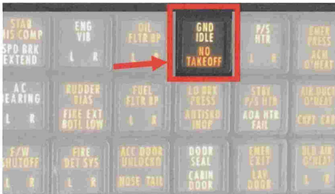
Figure 3 – The Cessna 560XL annunciator panel highlighting the "NO TAKEOFF" warning light.
