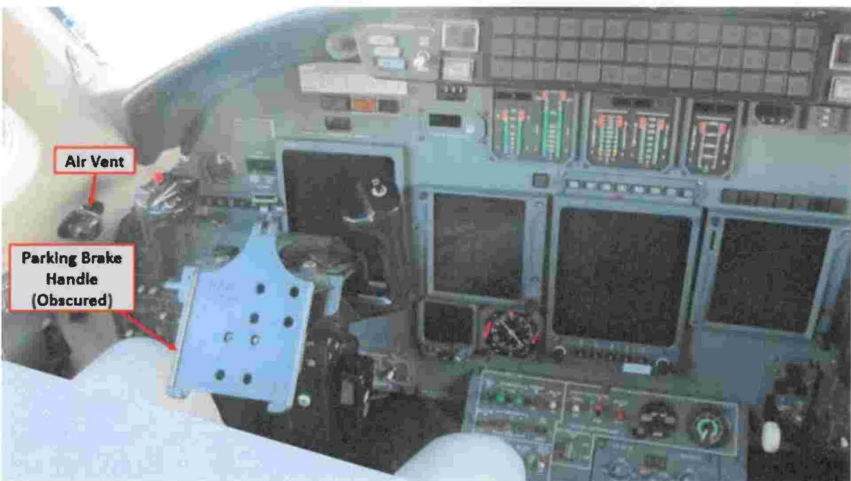
Figure 2 – Photograph showing how the location of the parking brake pull knob is obscured by the left-seat pilot and cockpit design.
